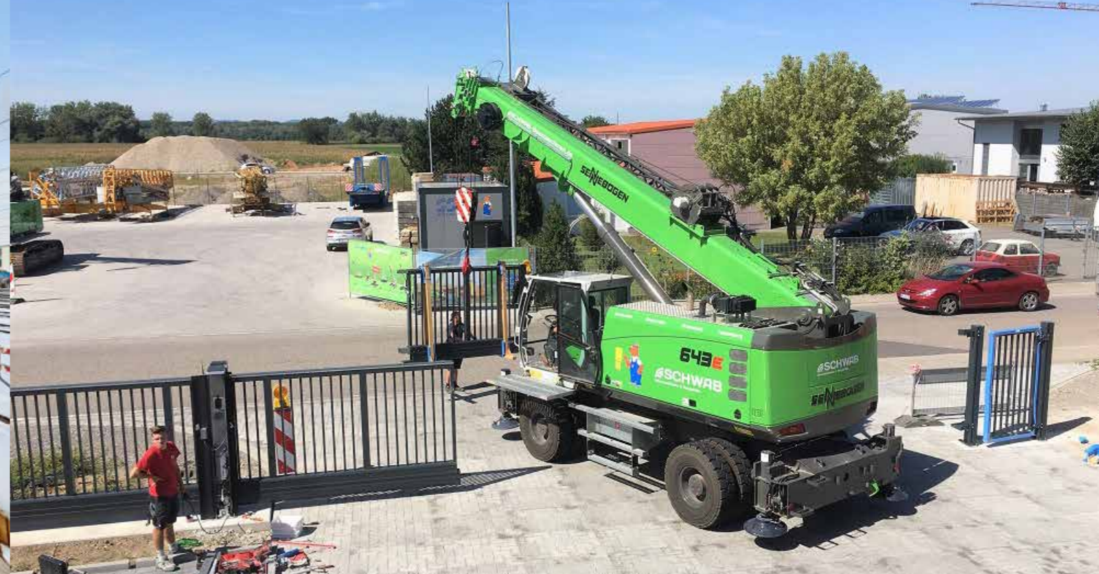
643 M - pick and carry operation; Germany 643 M - Pick and Carry Einsatz; Deutschland
